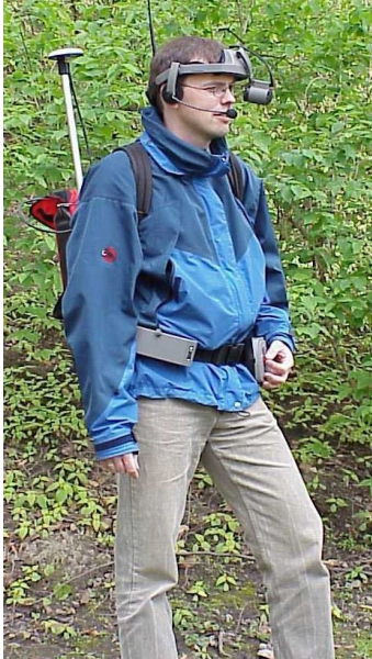
Fig. 3 Outdoor collection of vegetation data using a wearable computer that provides maps and map related information to the user. The interaction between user and application is based on various media: maps, text, symbolisation, and speech
