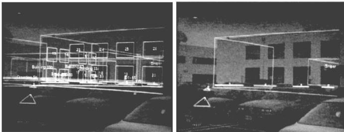
Figure 5. CAD model superimposed over real imagery
