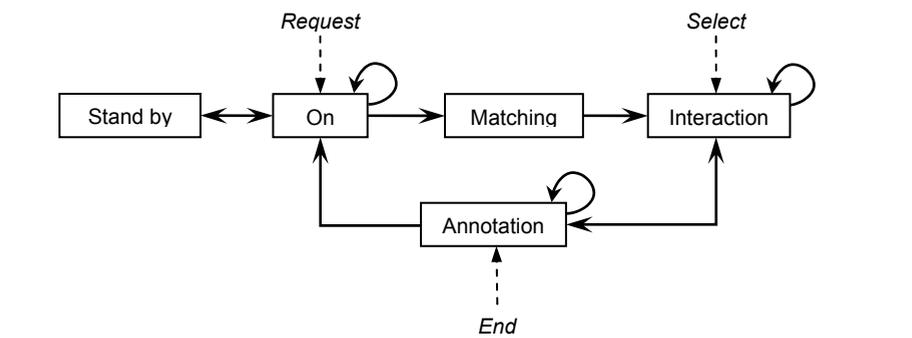
Figure 3. Scheme of operation of the portable system
