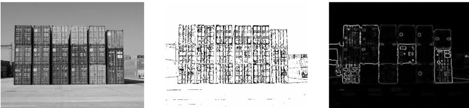
*Figure 6.* Original image (left) and border detectors. SUSAN (centre), Geusebroek (right)
