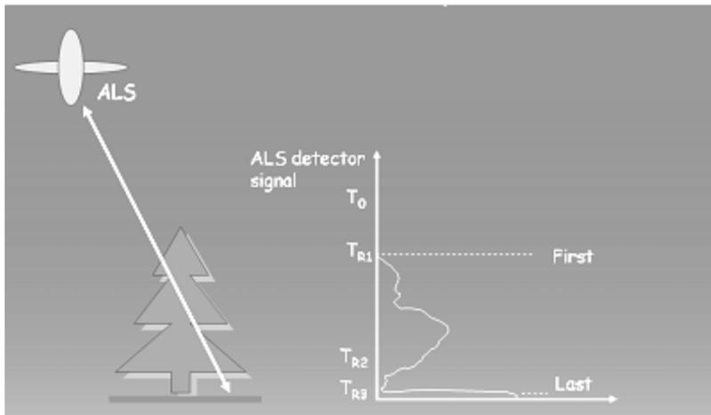
Figure 1. Interactions between the commercial Airborne Laser Systems (ALS) and the vegetation. Canopy height is estimated as the difference between the first and the last laser returns.
