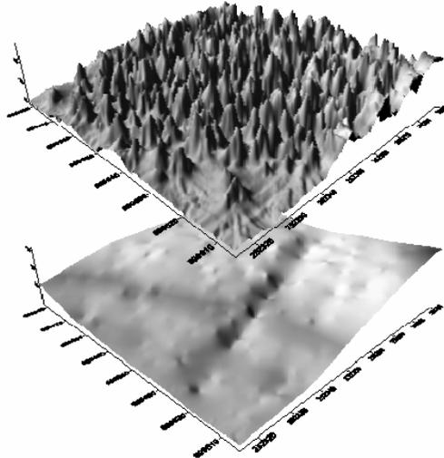
*Figure 7.* A Tree Canopy Model is created by the subtraction of the DTM from the original LiDAR first return. Example taken from plot 4 in Aberfoyle. The process of analysis will differentiate a tree canopy model and the underlying terrain.
