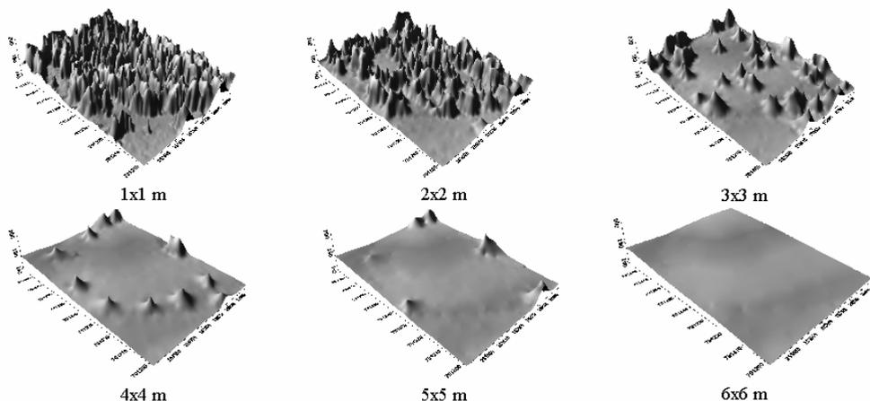
Figure 6. The filtering process of spurious ground hits is obtained by local minima in an iterative process using variable kernel sizes. Example obtained from plot 9 in Aberfoyle.
