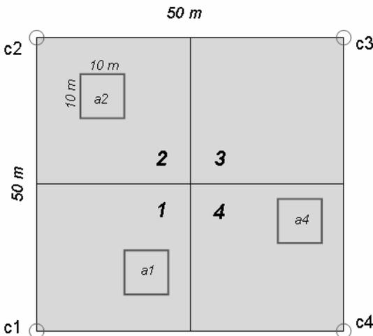
Figure 4. Configuration of the sample plots in the field. Plots are oriented to the magnetic north. Each corner is labelled with a 'c' and a number starting from the Southwest corner in sequence and finishing in the Southeast one. Each quadrant is labelled in the same sequence as the corresponding corners. Small plots of 10 x 10 metres are labelled with an 'a' and the number of the quadrant they lay in.
