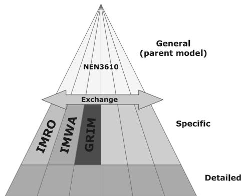
Figure 1: schematic representation of relationship between existing Dutch information models
