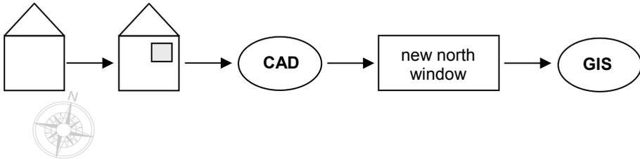
Figure 8: Only some characteristics of the building described in CAD are needed in GIS for simulation applications
