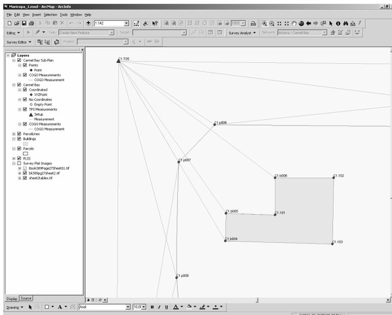
Figure 1: Including measurements in a GIS with ArcGIS Survey Analyst
