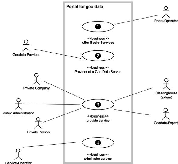
Figure 2: Use-Case Diagram for the system “Portal for Geo-Data” (Henrich, 2003)
