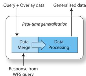
**Figure 2.** Real-time generalisation in DPSL can be divided into two phases: once the Value-added Service has added overlay data into the query, DPSL has to merge with spatial data requested from Data Integration Service. After this, DPSL processes this merged data and returns the generalised data.
