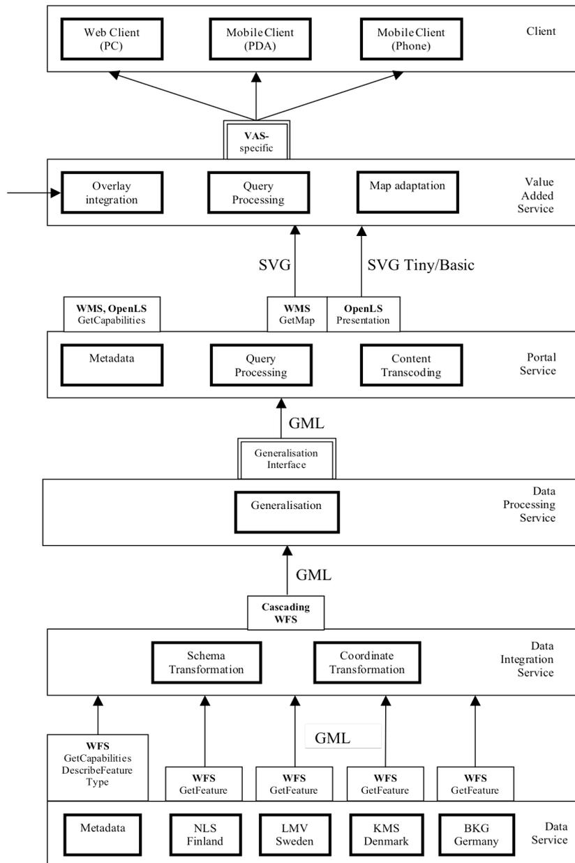
**Figure 1.** The detailed GiMoDig service architecture (Lehto and Sarjakoski, 2004). The arrows indicate the direction and encoding of the reply messages, while the arrows for requests have been omitted. The Value-added Service (VAS) layer can access external databases e.g. for retrieving Point of Interest (PoI) data. The access interfaces are based on Open Geospatial Consortium Specifications, except the VAS and Generalisation Interface, which have been developed in the project.
