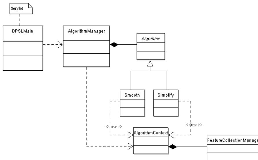
**Figure 3.** Class diagram of algorithms in Data Processing Service. The main class DPSLMain delegates the control of different algorithms to AlgorithmManager class. It has instances of all algorithms loaded into the system and it calls them with the use of AlgorithmContext class which contains all the parameters needed.
