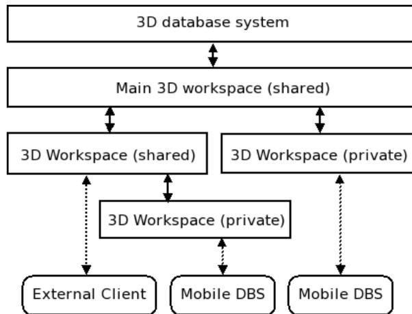
*Figure 1:* Structure of the version management system.
