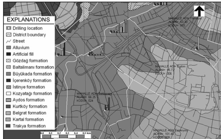
**Figure 4.** Presentation of the depth variables by using bar charts on the 2-dimensional GIS sheet.
