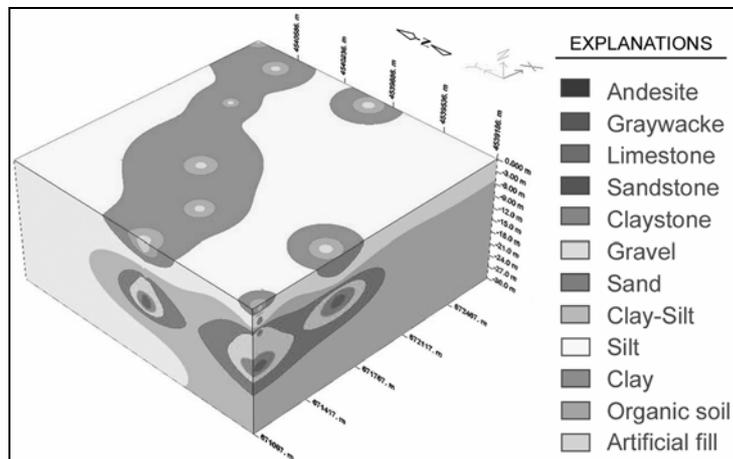
**Figure 5.** The variation of grain size with depth is seen on this real 3-dimensional volumetric diagram.
