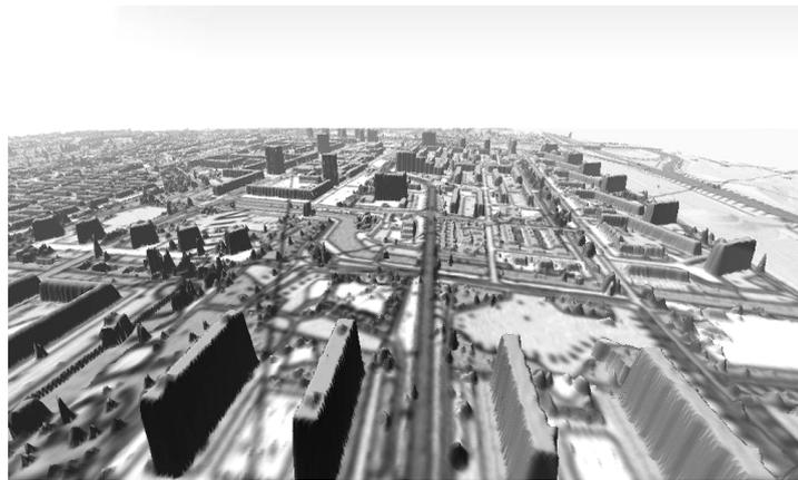
**Figure 1:** Draping the topographic map on top of unfiltered laserscan data
