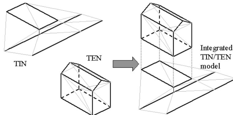
**Figure 3:** Combining 2.5D TIN and 3D TEN into a combined TIN/TEN model
