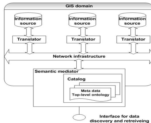
**Figure 1.** The role of domain oriented mediator in GeoNis architecture
