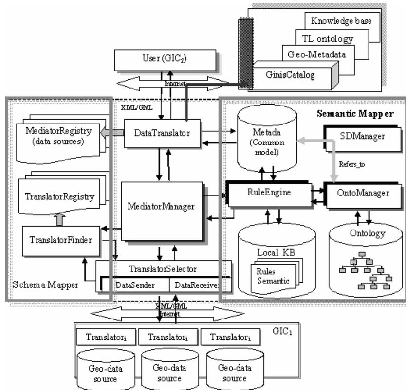
**Figure 2:** Architecture and role of Semantic Mediator in GeoNis.
