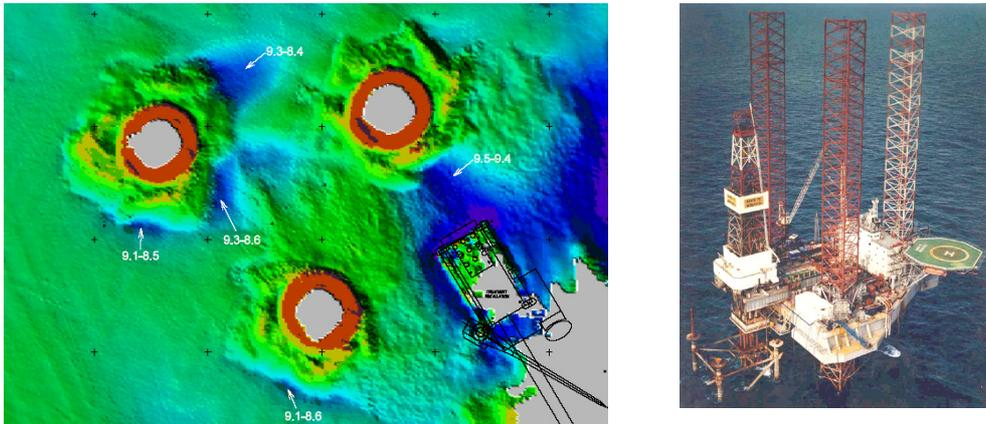
**Figure 1:** Bathymetry impression of jack-up rig footprints (up to 15 metres deep).
