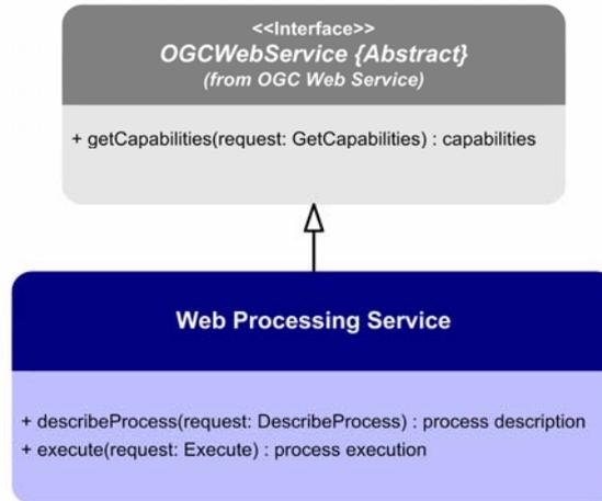
*Figure 1:* Web Processing Service interface definition
