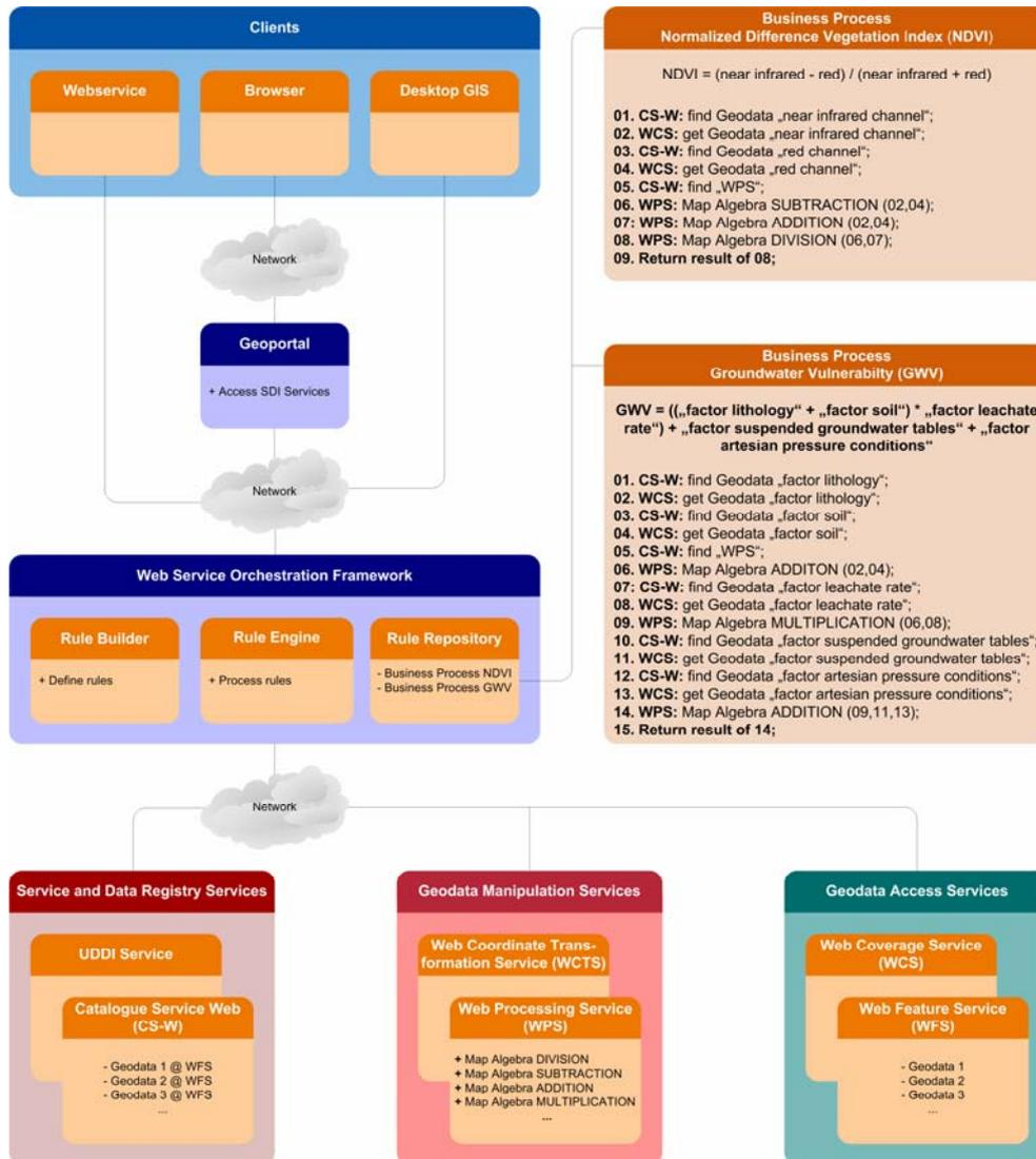
Figure 2: System architecture
