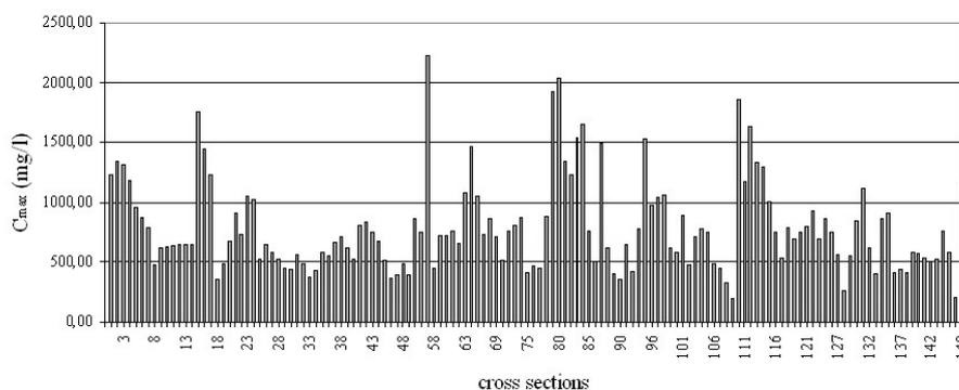
**Figure 6:** Maximum concentration in each cross-section in 100 m under the inlet ( $M=1000$  kg)
