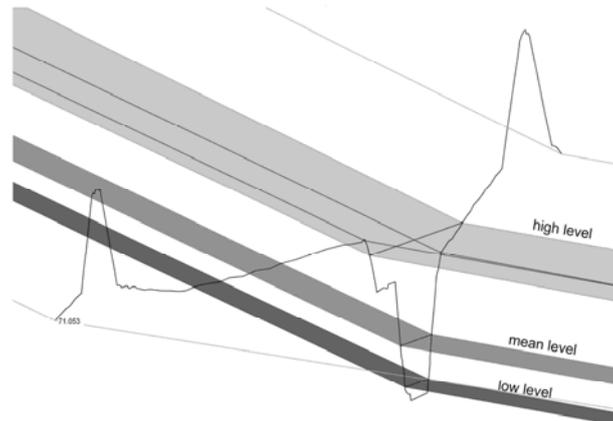
**Figure 3:** Different probability of the water levels at a cross section on the Berettyó River
