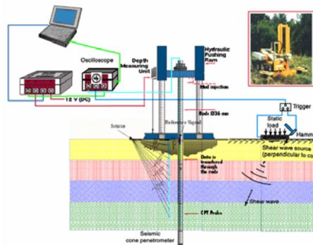
*Figure 2:* Schematic diagram of SCPT.
