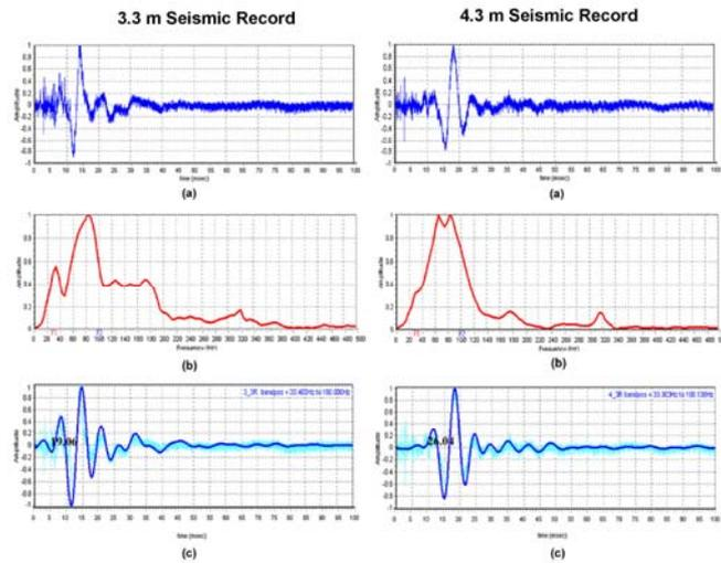
**Figure 3:** Seismic records obtained from two different levels. (a) Unfiltered seismic record. (b) Frequency spectrum of seismic signal. (c) Filtered seismic signal.
