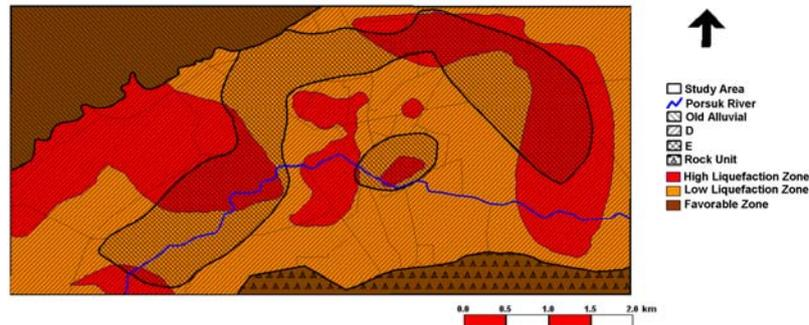
Figure 10: NEHRP classification and soil liquefaction map.
