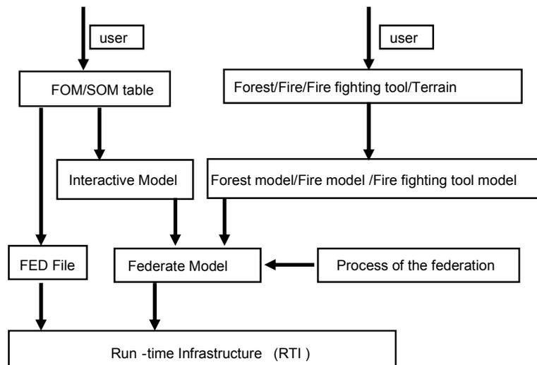
*Figure 2:* Design flowchart of the HLA federation
