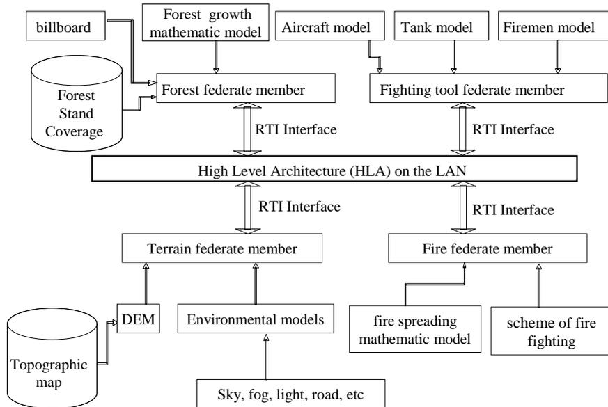
Figure 1: An HLA-based architecture of forest fire fighting system
