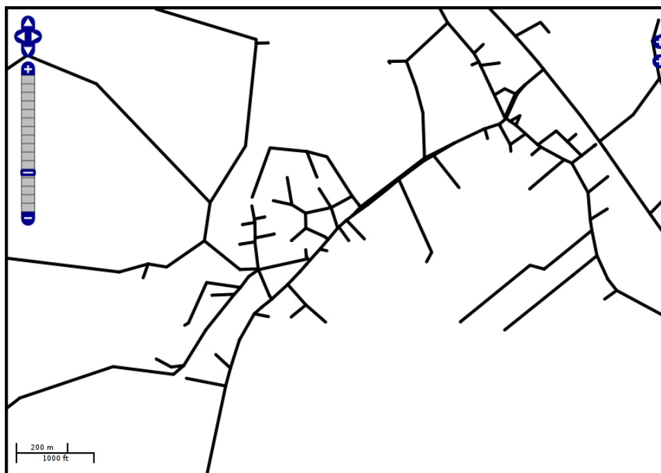
Figure 8: The Digiroad data after generalisation with the simplification operator.
