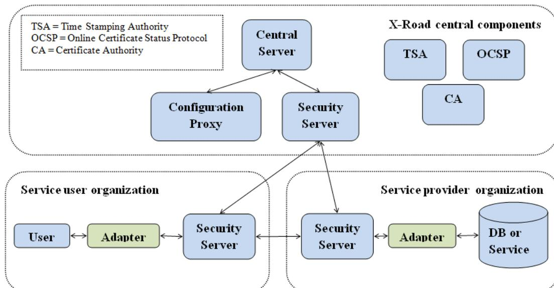
Figure 2: The request-response sequence in the X-Road platform.
