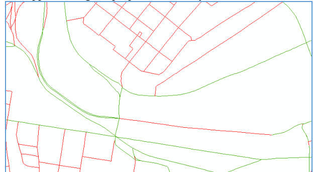
Figure 4. Part of the sample area after the thinning process is applied using the proposed hierarchy at scale 1:32K.
