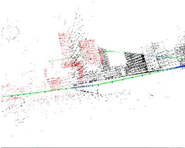
Figure 3: Orb-Slam2 localization and mapping on custom made city model
