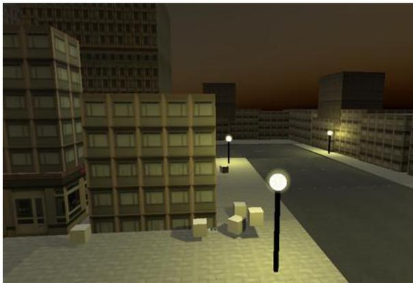
Figure 4: Unity3d custom-made city model for experiments (invisible cubes function as waypoints for automated flights for repeatability)
