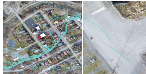
Figure 10: Zoomed center view of the drains and LCPA (left) and a closer view of the drains and waterflow (right), demonstrating the data resolution from the UAS
