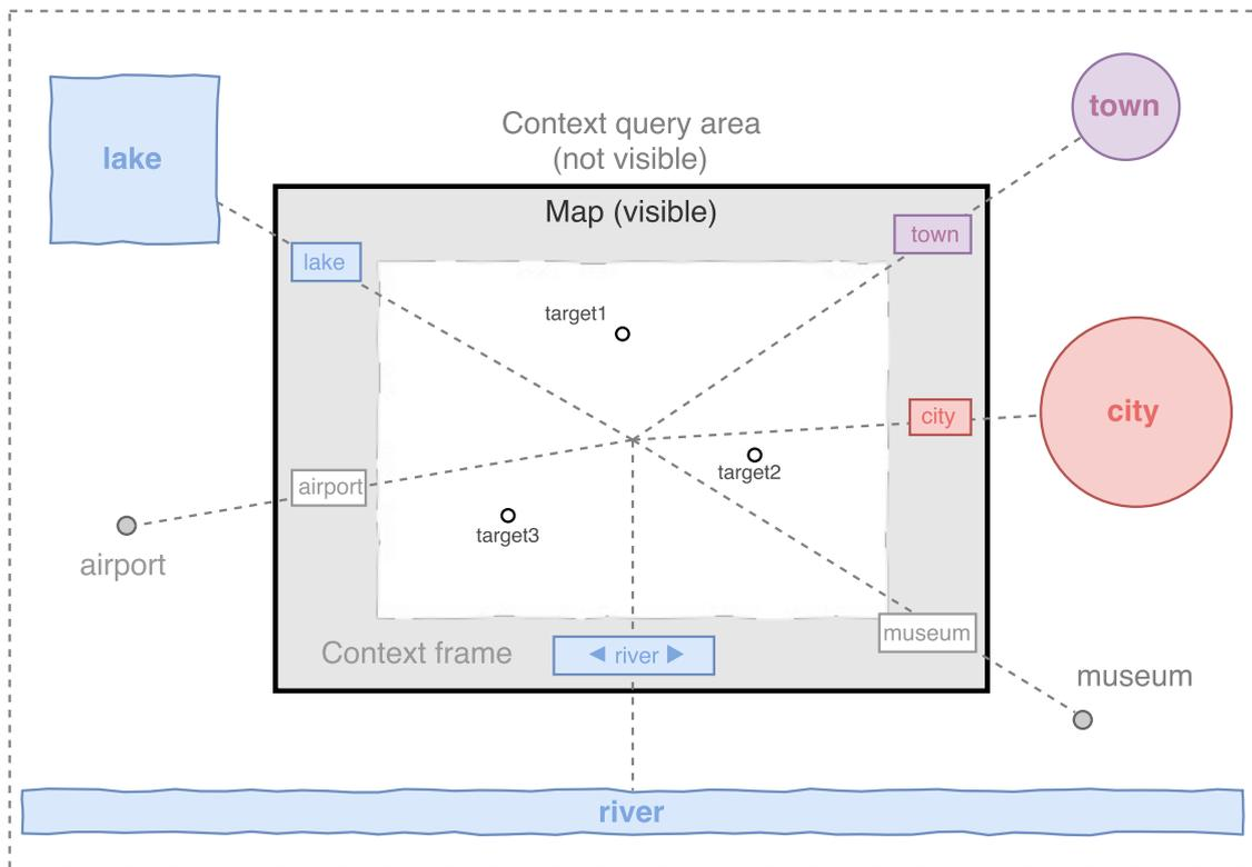
Figure 2: A schematic overview of the context frame, showing the map with some targets of interest (e.g. *target1*, *target2*, and *target3*), the context query area, and a set of notable objects. The notable objects must be contained in the context query area (not visible to the user), but not in the map (visible to the user). Depending on the scale, notable objects can be represented as points (e.g. airport and museum), as polygons (lake, city and town), and as polylines (river).
