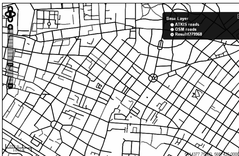
Figure 5: Screenshot of the application. The matching probability is represented by grayscale (black indicates high probability). In addition transferred (long dashed) and not matched (short dashed) features are visualized.
