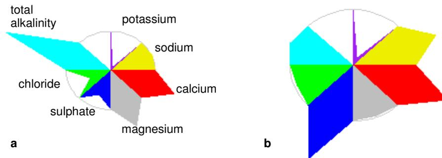
**Figure 1.** Maucha diagrams from sites in the Vaal River system, South Africa, a) C1H012 upstream of major pollution sources and b) C2H140 downstream of acid mine drainage and urban effluent sources. Drawn using an R script (DWA, 2011).
