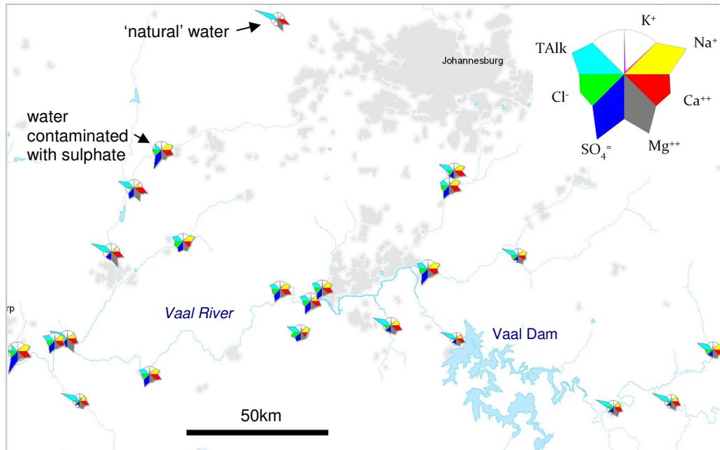
**Figure 2:** The river systems around Johannesburg, South Africa, with Maucha diagrams showing where sulphate ( $\text{SO}_4^-$ ) from mining operations has contaminated the surface water. Flow direction right to left. Generated in ArcGIS 9.2 using VBA script Maucha09.bas (DWA 2011).
