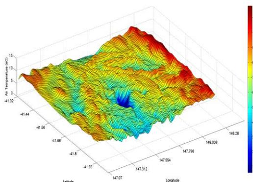
Figure 5 shows an example of the daily interpolated 3D spatiotemporal temperature surface for the entire South Esk sensor web.
