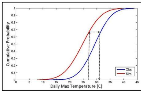
The scaling parameters that were obtained during the bias correction of model simulated historical precipitation and temperature were used to bias correct the future climate datasets.
