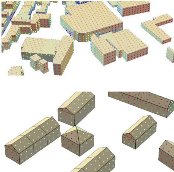
Figure 4: Global radiation on surfaces for one month computed for LOD 1 (top) and LOD 2 (bottom), normalized with respect to surface area (red indicates higher values, while blue refers to low values).
