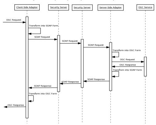
Figure 2: The request-response sequence in the X-Road platform.
