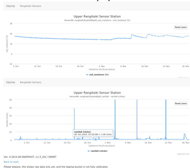
Figure 2: Raw sensor series visualized in a website from a SOS query.
