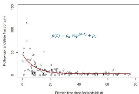
Figure 4. Temporal behaviour of landslide path dependency with an exponential decay
