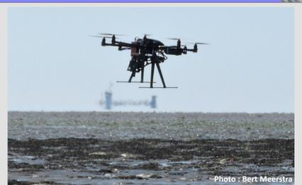
With an Unmanned Airborne Vehicle or drone, photos are taken of the mussel bed and computed into an ortho-photo with a detail of 2 cm. Current legislation limits the operation area for drone flying to 500 meters from the take-off point. To map a mussel bed longer than 1000 meters requires multiple take-off locations. Images with a detail of 1 mm can be acquired by flying at an altitude of 5 meters above ground level. This method is used to sample selected parts of the mussel bed.
