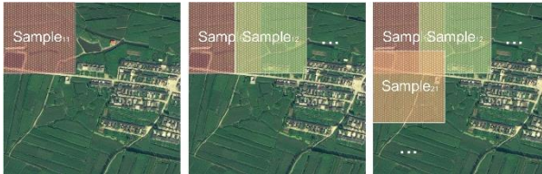
Figure 4: Overlapped Sampling Method (Here we take RS images as an example, GT-labels' sampling method is the same.)
